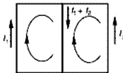
$$\left\{ \begin{array}{l} -U_1 + R_4 I_1 + R_1(I_1 + I_2) = 0 \\ U_2 - R_2 I_2 - R_3 I_2 - R_1(I_1 + I_2) = 0 \end{array} \right\} \Rightarrow \left\{ \begin{array}{l} (R_1 + R_4)I_1 + R_1 I_2 = U_1 \\ R_1 I_1 + (R_1 + R_2 + R_3)I_2 = U_2 \end{array} \right\} \Rightarrow \left\{ \begin{array}{l} 12I_1 + 10I_2 = 46 \\ 10I_1 + 12I_2 = 42 \end{array} \right\} \Rightarrow \left\{ \begin{array}{l} I_1 = 3 \text{ A} \\ I_2 = 1 \text{ A} \end{array} \right\}$$
