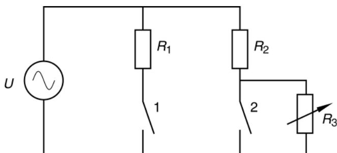
$$R_1 = 145 \Omega \quad R_2 = 100 \Omega \quad U = 230 \text{ V}$$
